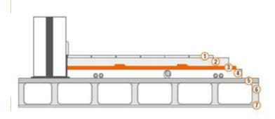
floor over a suitable elastic-resilient ester fibre coming from the recycling ving made the lightweight screed for on rating index to impact sound noise e frequency of 36 Hz such as AESSE
